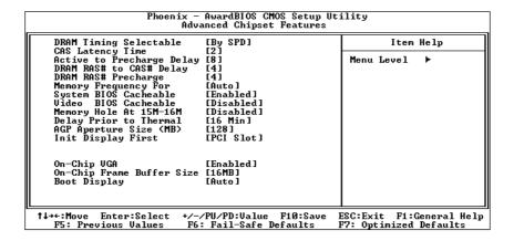
This section allows you to configure the system based on the specific features of the installed chipset. This chipset manages bus speeds and access to system memory resources, such as DRAM and the external cache. It also coordinates communications between the conventional ISA bus and the PCI bus. It must be stated that these items should never need to be altered. The default settings have been chosen because they provide the best operating conditions for your system.
