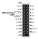
Attach your chassis HDD activity LED to this section of the header. Check for the correct polarity.
