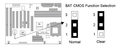
How to Remove the CMOS Setting
