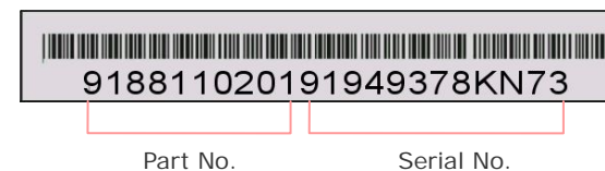
P/N: 91.88110.201 is part number, S/N: 91949378KN73 is serial number.
