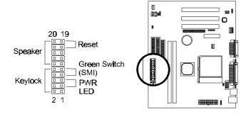
**Pins [3 & 5] Power LED lead** – Pins 3 and 5 connect to the power LED lead from the system's case. In case you case comes with a five-pin keylock & power LED connector, use the connector block marked as Keylock.
