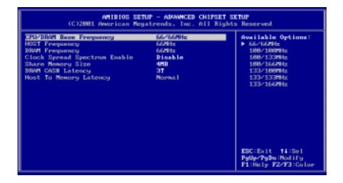
This section allows you to configure the system based on the specific features of the installed chipset. This chipset manages bus speeds and access to system memory resources, such as DRAM and the external cache. It also coordinates communications between the conventional ISA bus and the PCI bus. It must be stated that these items should never need to be altered. The default settings have been chosen because they provide the best operating conditions for your system.
