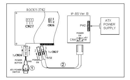
Connect the ATX power button switch to the pin 1 (power button) and pin 2 (+5VSB) of CN26 on the board. And connect the power cable from CN4 of backplane to CN27 of CPU card.
