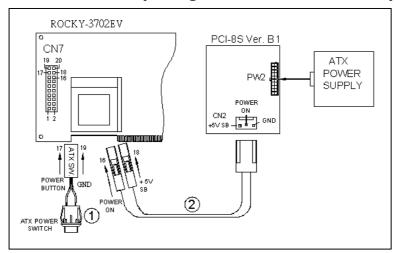
Connect the ATX power supply switch to the pin 17 (power button) and pin 19 (+5VSB) of CN7 (multi panel) on the board.
