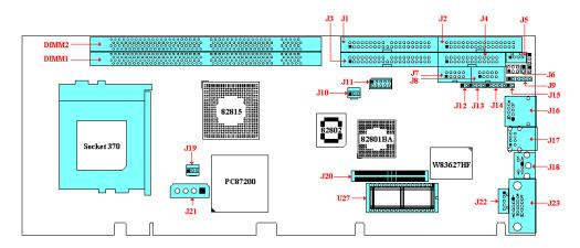
Figure 2-2 ROBO-679 Connector Locations
