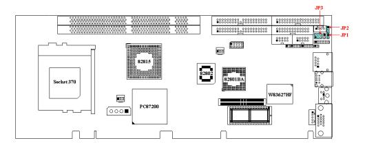
Figure 2-1 ROBO-679 Jumper Locations
