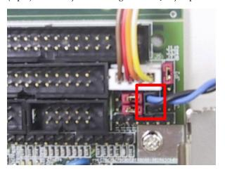
Step6: The figure below is the TOGGLE SWITCH, which is used to switch the ATX Power on/off for SBC. Usually the TOGGLE SWITCH is located on the chassis front panel. By pressing the switch button once, the power will be on, and press again to turn it off.
