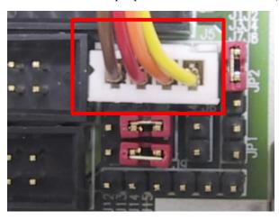
Step5: Connect TOGGLE SWITCH with J6 connector on ROBO-679. J6 connector (2-pin) is located just on the right side of JP3 jumper of ROBO-679.
