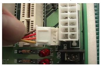
Step4: Please find the J5 4-pin header on the center part of ROBO-679 in white color. You will also see a mark with "J5" at the right top corner of J5 header. Connect the 4-pin power control cable with this J5 header.
