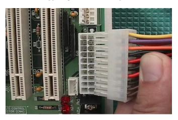
Step3: Use a 4-pin power cable to connect the CN4 (ATX P/S CONTROL CONNECTOR,4-pin) connector on the backplane.
