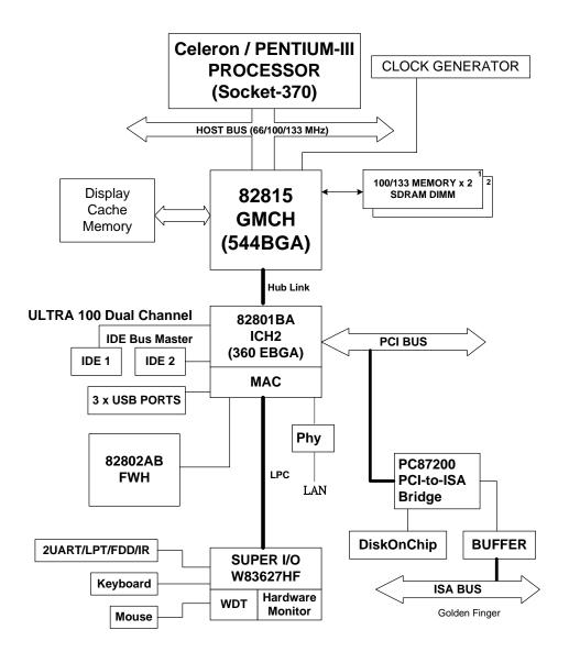
Figure 1-1 ROBO-679 System Block Diagram
