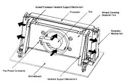
Figure 4 Airflow of fan/heatsink
