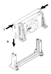
Figure 3. Slot 1 Pentium II CPU
