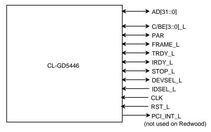
Figure 5 Video Controller PCI Signals
