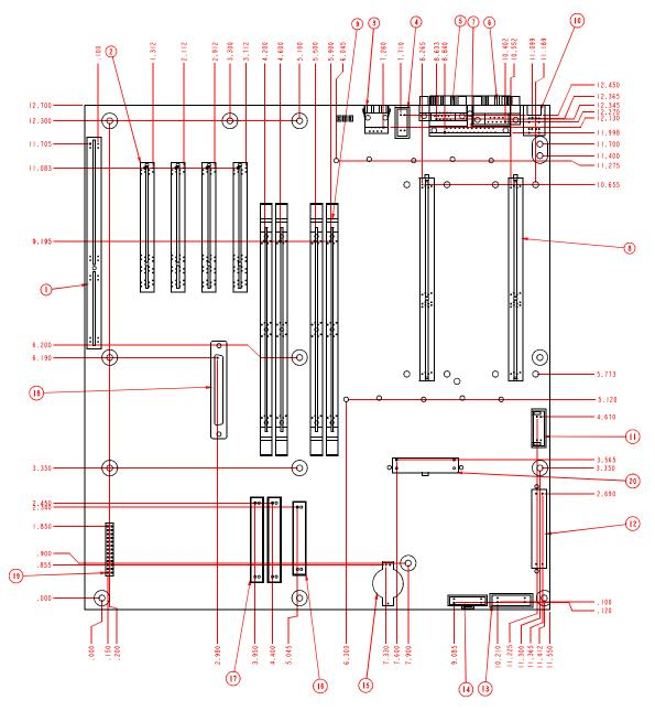
Figure 20 Baseboard Mechanical Diagram
