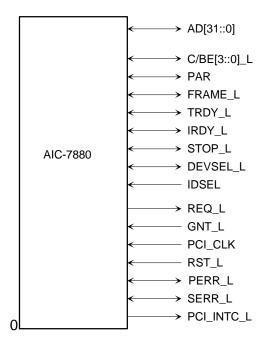
Figure 4 Embedded SCSI PCI Signals
