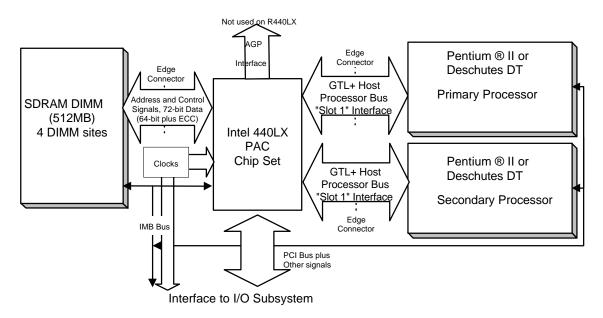
Figure 3 Processor/PCI Host Bridge/Memory Subsystem
