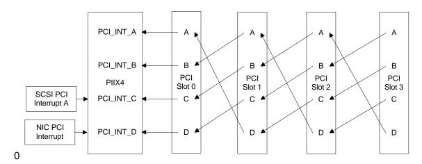
Figure 9 PCI Slot Interrupt Swizzle
