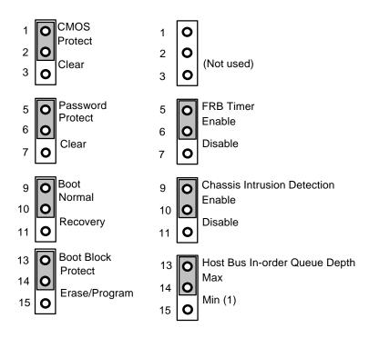
Figure 17 System Configuration Jumpers
