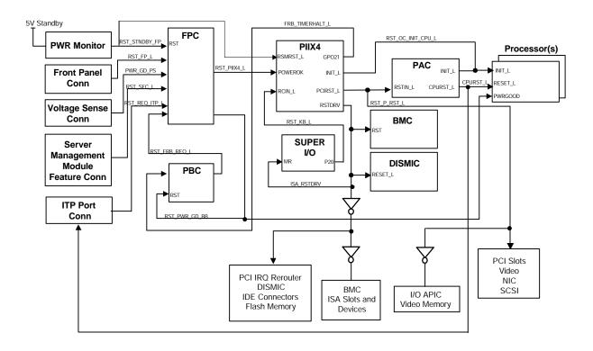
Figure 6 Reset Flow Diagram
