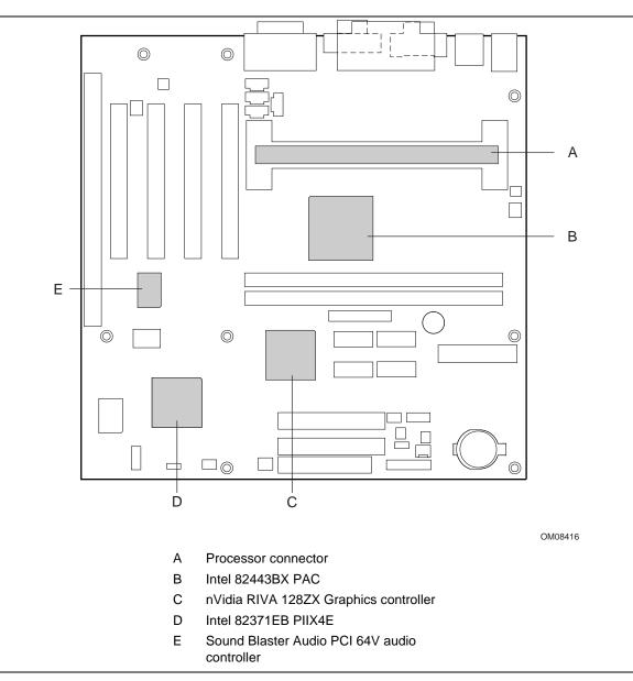
Figure 15. Thermally-sensitive Components
