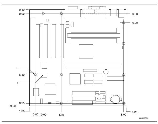
Figure 11. microATX Motherboard Dimensions
