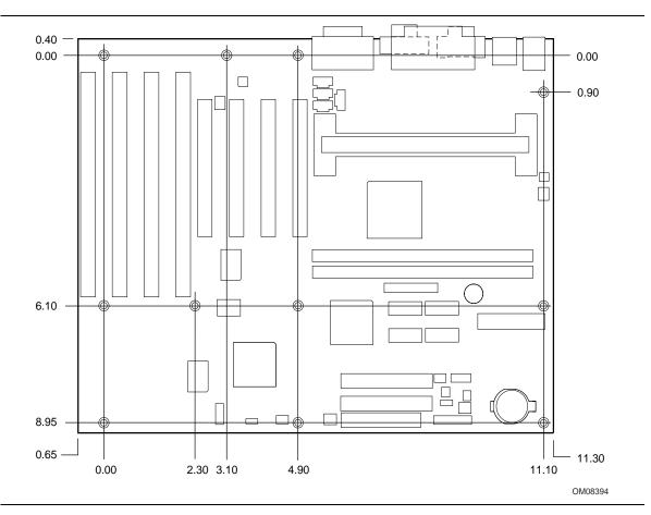
Figure 12. Full ATX Motherboard Dimensions
