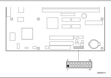
Figure 9. Front Panel I/O Connectors
