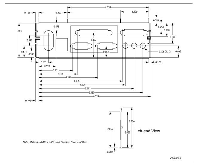
Figure 13. Back Panel I/O Shield Dimensions (Intel ATX/microATX Chassis)
