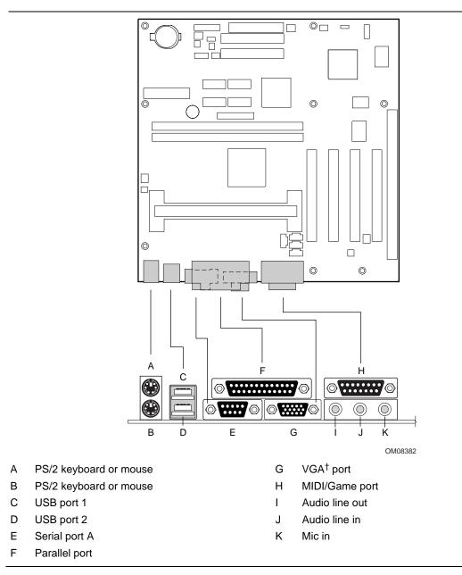
Figure 4. Back Panel I/O Connectors
