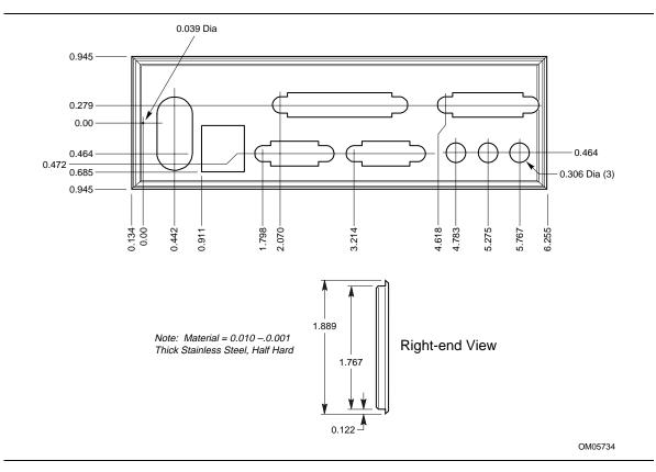
Figure 14. Back Panel I/O Shield Dimensions (ATX/microATX Chassis-Independent)
