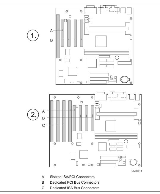
Figure 8. Add-In Board Connectors
