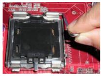
1.Please turn off the power and unplug the power cord before installing the CPU. Use index finger and thumb to raise the metal lever so it is separated from the bottom steel shell grip hook.
