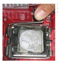
Press the metal lever so it is secured in the bottom steel shell grip hook.
