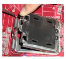
2.Use index finger to lift the top steel shell.
