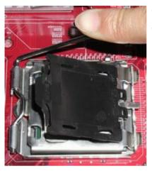
4.Use index finger and thumb to press down the metal lever. The cap will be pushed up by the CPU. This may also be done by removing the lid beforehand.
