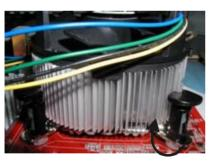
9. Gently rotate the cap clockwise 1/4 turn to fasten the heatsink onto the Sapphire motherboard.
