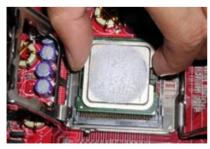
3.Use index finger and thumb to place the CPU onto the socket (Look for the gold arrow. The gold arrow should point towards the lever pivot).
