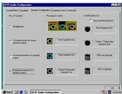
7. 2/4/6 channel speaker configuration setting
