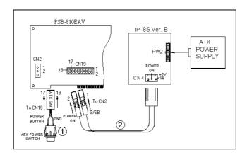
Connect the ATX power button switch to the pin 17 (power button) and pin 19 (+5VSB) of CN19 on the board. And connect the power cable from CN4 of backplane to CN2 of CPU card.
