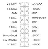
Fig. 5 ATX Power Supply Connector
