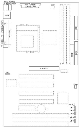
Fig 3 Connector Location
