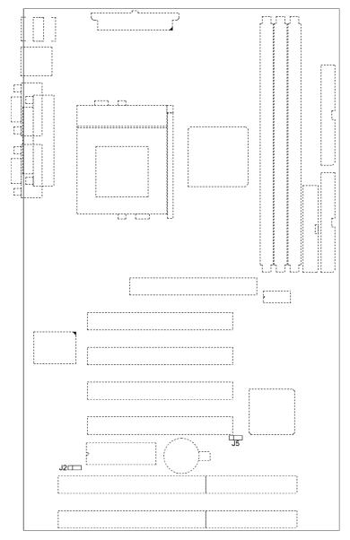
Fig. 2 Jumper Location of the mainboard
