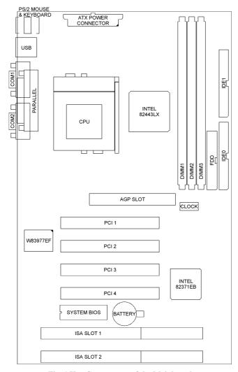
Fig. 1 Key Components of the Mainboard
