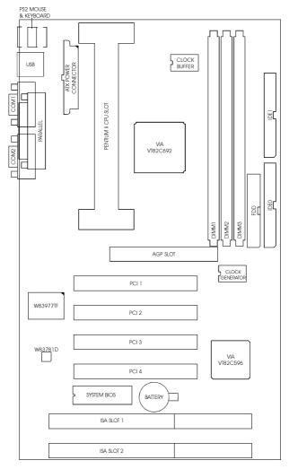
Fig. 1 Key Components of the Mainboard
