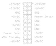
Fig. 5 ATX Power Supply Connector
