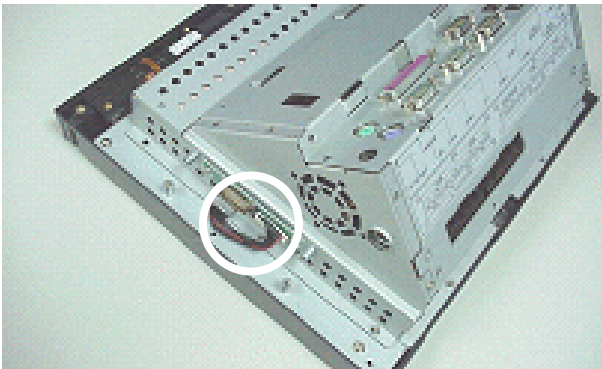
j. Disconnect the keypad cable
