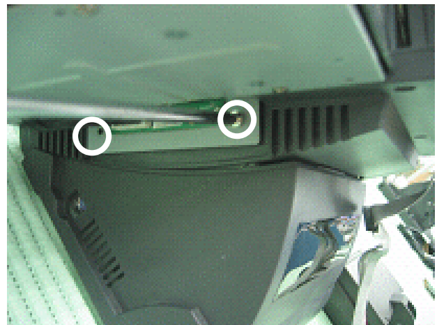
f. Tighten the two screws so the keypad can be fully connected to the system.
