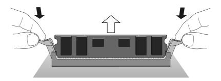
Press the tabs on both of the socket's end clips at the same time. This releases the DIMM and lifts it partly out of the socket.
