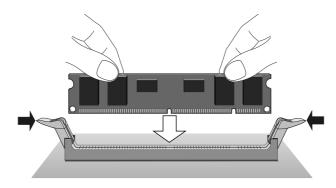
The DIMM is inserted vertically and held in place by the clips at each end.
