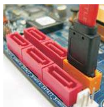
Connect the SATA data cable to the orange SATAII connector (SATAII_6 (PORT3.1))
