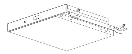
Fit the CD/DVD Interface PCB to the drive connector and secure it using two M2 x 6mm screws through the plastic bushes into the drive body (see diagram).
