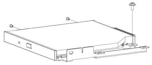
Re-install the Drive Baseplate into the chassis taking care not to trap any of the wiring, and secure using the two M3 x 6mm screws removed earlier. Check that the drive door is clear of the chassis and tighten the screws.
