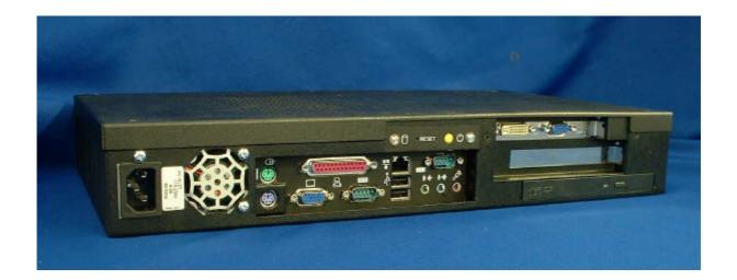
The PE3M is a powerful slim-line Intel Pentium P4-based Personal Computer (PC) specifically designed to drive large plasma and other large displays panels. The unit is self-contained requiring as a minimum, only a power connection and a display. The applications are not limited to display applications: it may be used as a general purpose PC.
