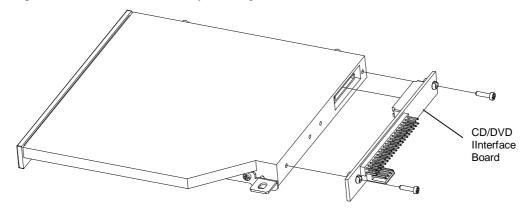
Fit the drive and PCB assembly to the Removable-Drive Baseplate, so that the tab on the CD/DVD Mounting Bracket engages with that on the Baseplate.
