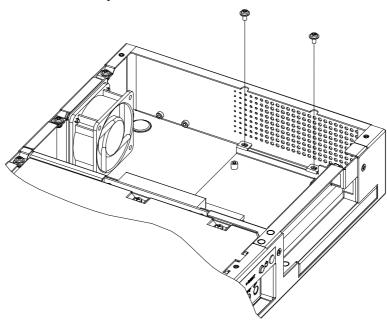
Using two M2 x 3mm cap-head screws, fix the CD/DVD Mounting Bracket to the cut away side of the drive (see diagram).
