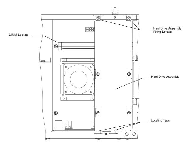
Remove the hard drive assembly as follows:
