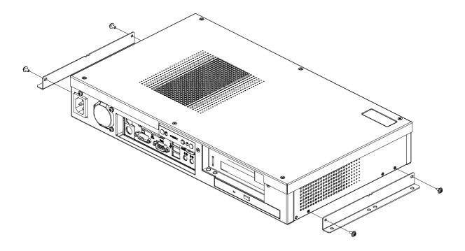
Assemble the PE3M to the display using four M4 x 6mm screws.
