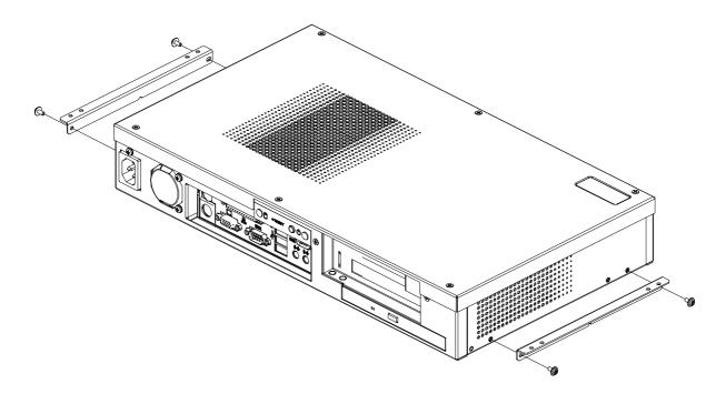
Fit the right-angle AC power connector to the PC. *DO NOT CONNECT THE AC POWER AT THIS STAGE*. Assemble the PE3M to the display using four M3 x 6mm screws.
