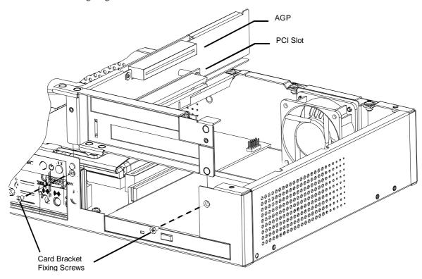
Remove the two M3 countersunk-head screws on the front face of the chassis (in line with the upper [AGP] card bracket).
