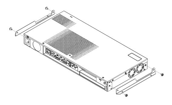
Assemble the PE2M to the display using four M3 x 6mm screws.
