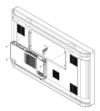
Fit the right-angle AC power connector to the PC. DO NOT CONNECT THE AC POWER AT THIS STAGE.
