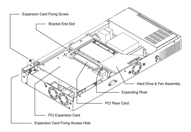
Remove the hard drive assembly as follows:
