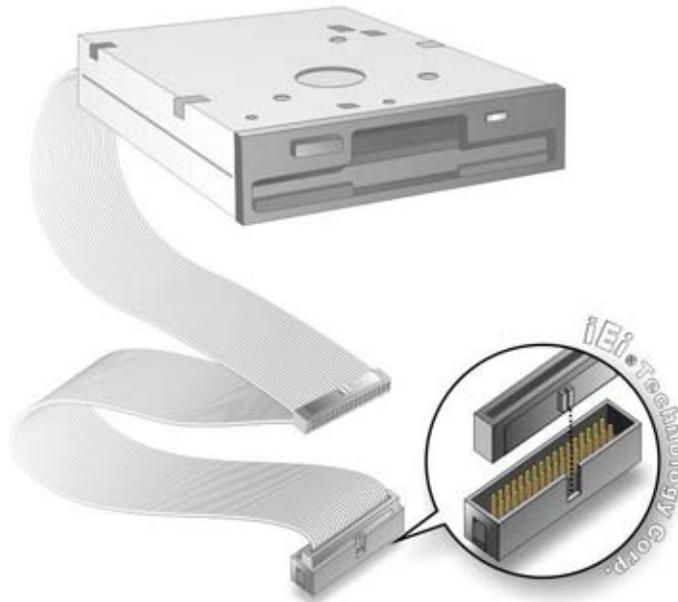
**Figure 4-9: FDD Cable Connection**
