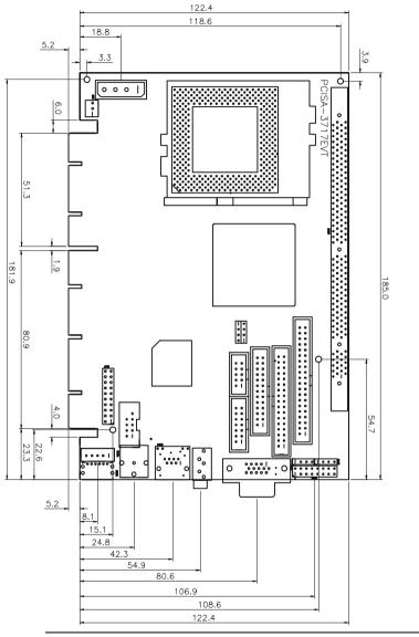
PCISA-3717EVT Socket 370 Celeron™ & Pentium III ® with Ethernet , VGA( Dual Display ) , TV-Out ,Audio Board
