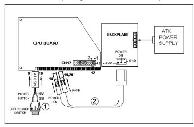
Connect the ATX power supply switch to the pin 9 (power button) and pin 19.20 (+5VSB) of CN17 on the board.
