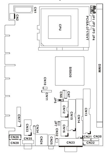
PCISA-3717EVT Socket 370 Celeron™ & Pentium III ® with Ethernet , VGA( Dual Display ) ,
