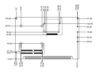
Figure 1.2: Board layout: dimensions (solder side)
