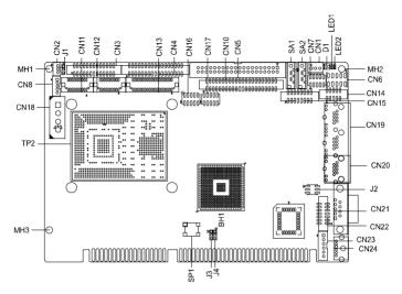
Figure 2.1: Jumper & Connector Locations
