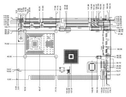
Figure 1.1: Board layout: dimensions (component side)
