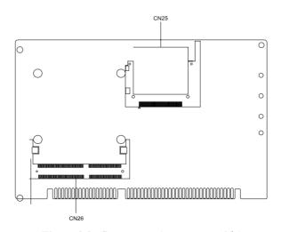
Figure 2.2: Connectors (component side)
