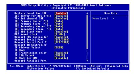
Figure 3-5: Integrated Peripherals Setup
