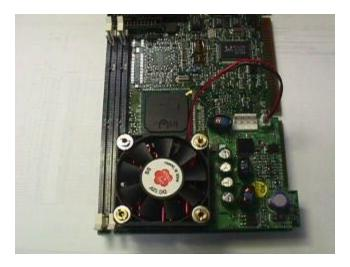
Figure 3-5: Affixing the CPU/fan assembly to the board
