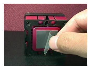
Figure 3-2: Peeling off the thin plastic coating of the CPU fan
