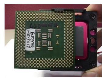
Figure 3-3: Pushing the Coppermine/Celeron  $^{\text{TM}}$  into the frame
