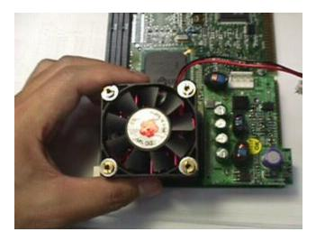
Figure 3-4: Placing the CPU/fan assembly on the board
