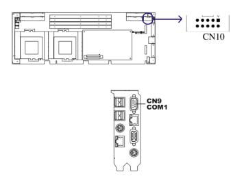
The PCA-6277 offers two serial ports, CN9 as COM1 and CN10 as COM2. These ports can connect to serial devices, such as a mouse or a printer, or to a communications network.
