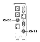
Two 6-pin mini-DIN connectors (CN11 and CN33) on the card mounting bracket provide connection to a PS/2 keyboard and a PS/2 mouse, respectively. CN11 can also be connected to an adapter cable (P/N: 1700060202, available from Advantech) for connecting to both a PS/2 keyboard and a PS/2 mouse.
