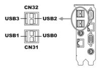
The PCA-6277 provides four ports of USB (Universal Serial Bus) interface, which gives complete Plug & Play and hot swapping for up to 127 external devices. The USB interface complies with USB Specification Rev. 1.0 and is fuse-protected.
