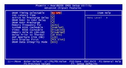
Figure 3.4: Advanced chipset features screen
