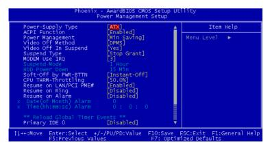
Figure 3.9: Power management setup screen (1)
