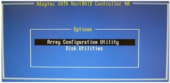
Figure 9.1: RAID Setup initial screen
