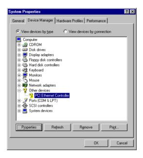
3. In the "PCI Ethernet Controller Properties" window, select the "Driver" tab. Then click on "Update Driver...".
