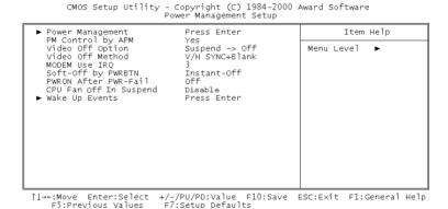
Figure 3-6: Power management setup screen
