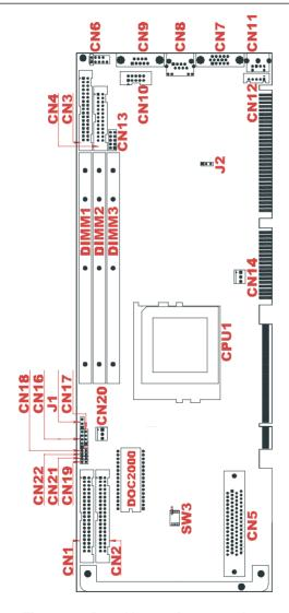
Figure 1-2: Board layout: jumper and connecter locations
