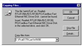
10. When the "Insert Disk" window appears, insert the utility CD into the CD-ROM drive. Then click on "OK".
