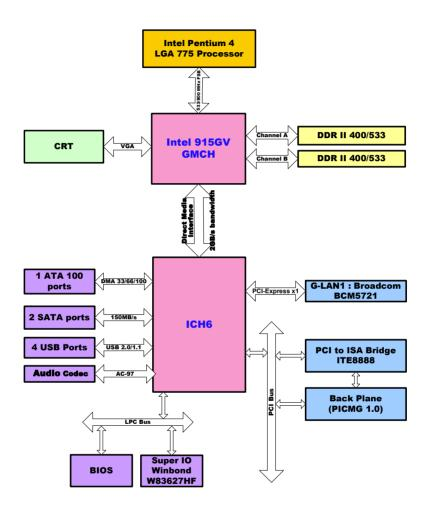
Figure 1.2: Block Diagram
