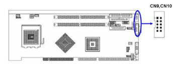
The PCA-6009 offers two serial ports, CN9 as COM1 and CN10 as COM2. These ports can connect to serial devices, such as a mouse or a printer, or to a communications network.
