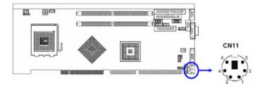
One 6-pin mini-DIN connectors (CN11) on the card mounting bracket provide connection to a PS/2 keyboard or a PS/2 mouse, respectively. CN11 can also be connected to an adapter cable (P/N: 1700060202, available from Advantech) for connecting to both a PS/2 keyboard and a PS/2 mouse.
