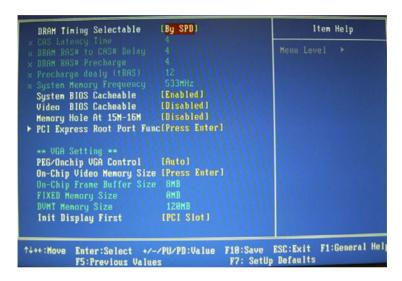
Figure 3.4: Advanced chipset features screen
