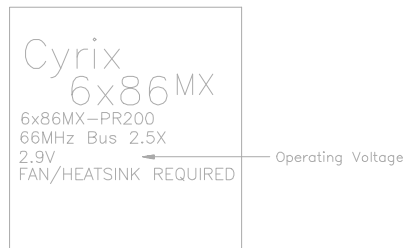
Fig. 2g CPU Description (Top Side)
