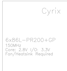
Fig. 2f CPU Description (Top Side)
