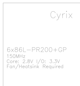
Fig. 2f CPU Description (Top Side)
