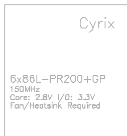
Fig. 2f CPU Description (Top Side)
