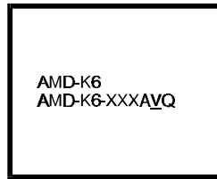
V (Identifier for Operational Voltage) N 3.1-3.3V Core/3.135-3.6V I/O L 2.755-3.045V Core/3.135-3.6V I/O
