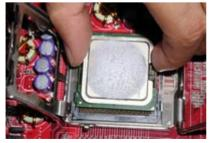
3.Use index finger and thumb to place the CPU onto the plastic body (look for the gold arrow, the gold arrow should point away from the lever pivot).
