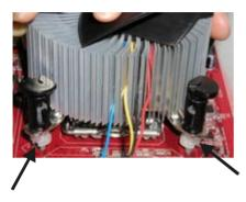
7. Align the fastener tips with the motherboard hole pattern, insert the fastener tips into the holes, guilding the wires to avoid pinching. the fasteners will slide through the motherboard holes with no insertion force.
