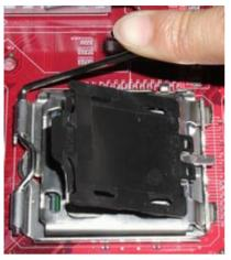
4. Press the metal lever down to force the cap to be pushed up by the CPU; This may also be done by removing the lid beforehand.
