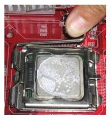
5. Press the metal lever down and hook it to the bottom steel shell grip hook.
