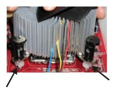
7. Align the fastener tips with the Sapphire motherboard hole pattern, insert the fastener tips into the holes, guiding the wires to avoid pinching. The fasteners will slide through the motherboard holes with no insertion force.
