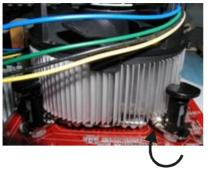
9. Gently rotate the cap clockwise 1/4 turn to fasten the heatsink onto the Sapphire motherboard.
