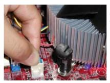
10. Lastly, attach the fan wire connector to the 4 pin fan header connector on the Sapphire motherboard labeled CPU FAN.
