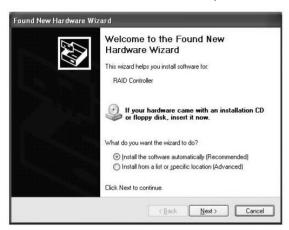
2. Insert the bundled driver CD into your CD-ROM drive and select "ATI Chipset\ATI\_Raid Driver"installation bar on the dialogue window to begin the driver and software installation (Please follow the instructions to finish the installation).
