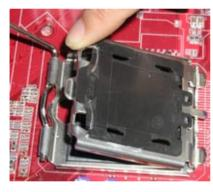
2.Use the index finger to lift the top steel shell.
