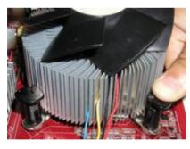
8.Engage the fasteners' caps. Apply thumb pressure to the top of each of the 4 fastener caps. (there is no specific order of engagement). You will hear a "click" upon full engagement.
