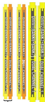
DIMM1 & DIMM2: Dual Channel 1 DIMM3 & DIMM4: Dual Channel 2
