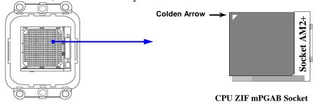
When you put the CPU into the ZIF socket, No force require to insert of the CPU, then press the level to Locate position slightly without any extra force.
