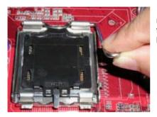
1.Use index finger and thumb to move metal lever so it is separated from the bottom steel shell grip hook.
