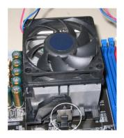
Step2. Locate the Fix lever, Safety Hook and the Fixed Bolt. Lift up the intensive fixed lever.
