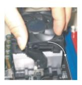
Step4. Make sure the safety hook completely clasps the fixed bolt of the retention mechanism.
