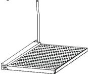
2. Look for the gold arrow. The gold arrow should point towards the lever pivot. The CPU can only fit in the correct orientation.
