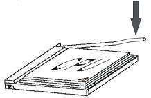
5. When you are installing the CPU,make sure the CPU has a heat sink and a cooling fan attached on the top to prevent overheating. If you do not have the heat sink and cooling fan, contact your dealer to purchase and install them before turning on the computer. please follow below steps to install the CPU cooler.
