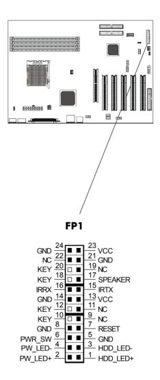
The motherboard provides one AGP slot, five 32-bit PCI bus slots.
