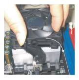
Step4. Make sure the safety hook completely clasps the fixed bolt of the retention mechanism.
