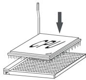
2. If the CPU is correctly installed, the pins should be completely embedded into the socket and can not be seen. Please note that any violation of the correct installation procedures may cause permanent damages to your mainboard.
