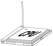
4. Press the CPU down firmly into the socket and close the lever. As the CPU is likely to move while the lever is being closed, always close the lever with your fingers pressing tightly on top of the CPU to make sure the CPU is properly and completely embedded into the socket.
