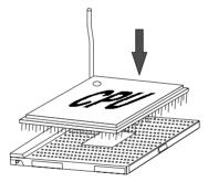
2. If the CPU is correctly installed, the pins should be completely embedded into the socket and can not be seen. Please note that any violation of the correct installation procedures may cause permanent damages to your mainboard.
