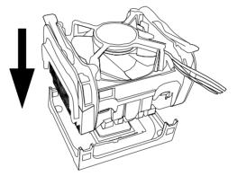
6. Use one end of the clip to hook the latch of the CPU sliding plate and then hook the other three latch to fix the cooling fan set. At last, connect the fan to the power supply connector provided on your mainboard.
