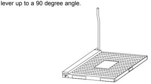
2. Look for the gold arrow. The gold arrow should point towards the lever pivot. The CPU can only fit in the correct orientation.
