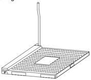
2. Look for the gold arrow. The gold arrow should point towards the lever pivot. The CPU can only fit in the correct orientation.
