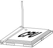
4. Press the CPU down firmly into the socket and close the lever. As the CPU is likely to move while the lever is being closed, always close the lever with your fingers pressing tightly on top of the CPU to make sure the CPU is properly and completely embedded into the socket.
