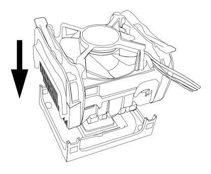
6. Use one end of the clip to hook the latch of the CPU sliding plate and then hook the other three latch to fix the cooling fan set. At last, connect the fan to the power supply connector provided on your mainboard.
