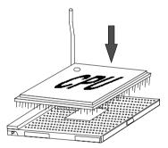
If the CPU is correctly installed, the pins should be completely embedded into the socket and can not be seen. Please note that any violation of the correct installation procedures may cause permanent damages to your mainboard.
