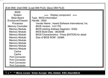
**Note:** The DMI utility must be run in real mode without the EMM386 memory manager loaded.
