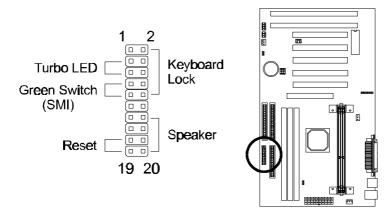
**Pins [3 & 5] Turbo LED switch** - The Turbo function is not supported by this mainboard. Therefore, the Turbo LED will always remain lit as long as the system power is on.
