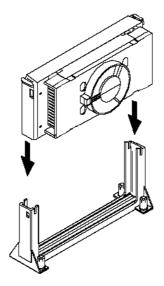
2. Seat the CPU firmly into the slot until the two tabs on the CPU click outwards to lock the CPU in place.
