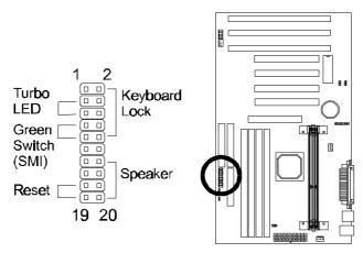
**Pins [3 & 5] Turbo LED switch** - The Turbo function is not supported by this mainboard. Therefore, the Turbo LED will always remain lit as long as the system power is on.
