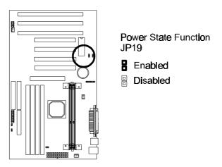
"PWRON After PWR-Fail" in the Power Management Setup must be set accordingly. Refer to pages 43 and 45 for more information.
