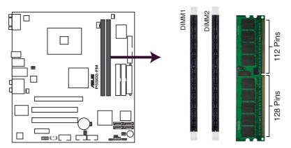
P5SD2-FM 240-pin DDR DIMM Sockets
